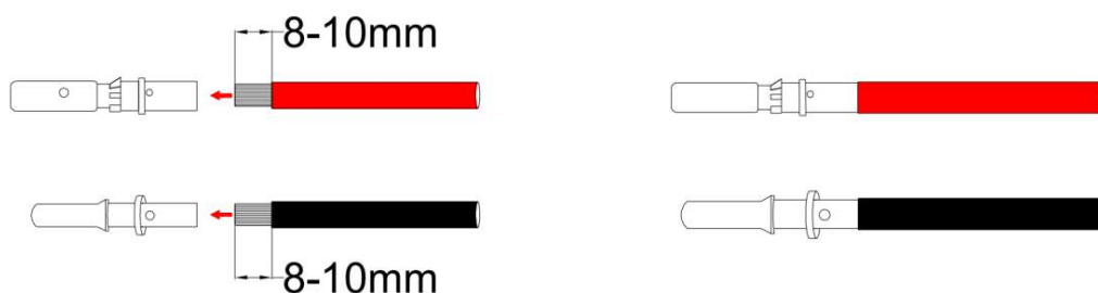
Figure 4.6-6 Prepare BAT-inverter cables
